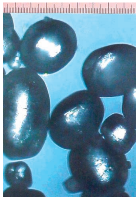
Figure 1. Microscopic picture of I7 from toluene crystallization. Scale: distance between short bars corresponds to 13.2 \mu\text{m} . Rounded edges caused by attrition.
